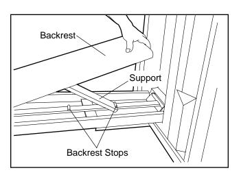
To adjust the backrest to the level position, first raise the backrest slightly. Pivot the end of the support in the direction shown by the arrow. Lower the backrest onto the hench
